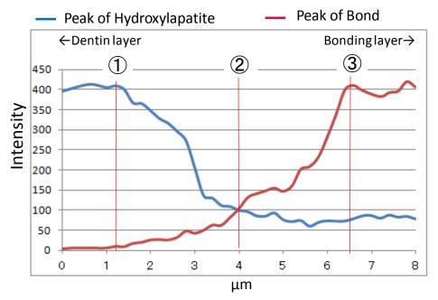
Fig. 28 Raman analysis of PALFIQUE UNIVERSAL BOND
