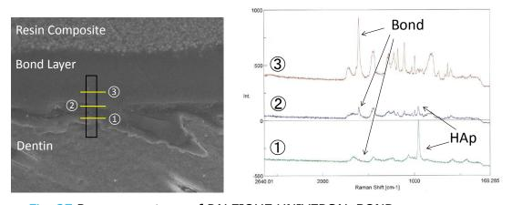
Fig. 27 Raman spectrum of PALFIQUE UNIVERSAL BOND
