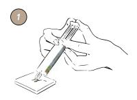
Press the syringe with two hands and squeeze out equal volume units of base (yellow) and catalyst (white) material in a 1:1 ratio on the mixing pad.
